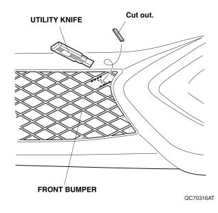
24. Route the heater harness through the front bumper as shown, then reinstall the front bumper with the help of an assistant.
