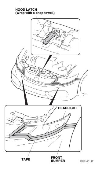
• Remove the 4 self-tapping screws, 10 clips, and 2 bolts.
