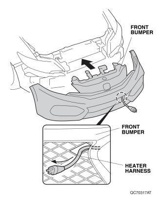
25. Using one black wire tie, secure the heater harness to the front bumper.
