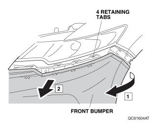
• With the help of an assistant, remove the front bumper (four clips and unplug the vehicle connectors). Place the front bumper on a blanket to prevent damage.
