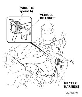
13. Route the heater harness as shown. Secure the heater harness to the fan shroud rib with one wire tie at the white mark (point B).
