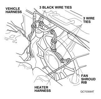
16. Route the heater harness under the vehicle frame as shown.
