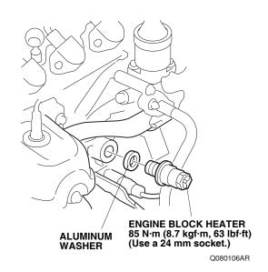
11. Plug the connector end of the heater harness into the engine block heater. Make sure the heater harness connector is fully seated in the engine block heater.
