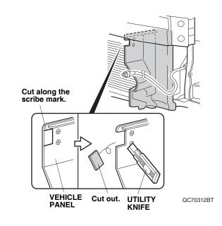
20. Using a pushpin, pierce the two scribe marks on the vehicle panel at the location shown. While wearing eye protection, drill the two pierced marks with a 3 mm drill bit, then enlarge the holes with a 5 mm drill bit as shown. Remove any burrs.
