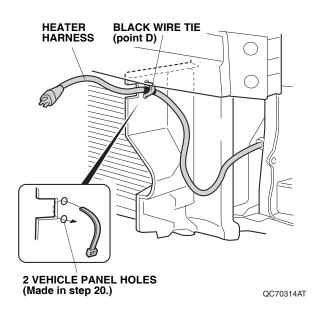
22. Bundle up the excess heater harness, and secure it to the vehicle panel hole with one black wire tie.
